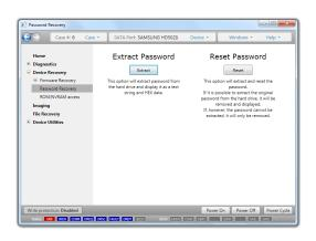
Identify and/or Remove unknown passwords regardless of setting (Master or User) or security level (High or Maximum).
