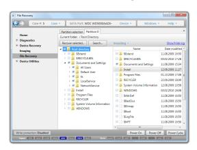
The Atola Insight File Recovery Engine extracts files from badly damaged hard drives, even in cases where all partitions are lost. It does this by scanning a hard drive's entire platter area to identify possible system file structures (such as MFT) and then recovering the original file and folder structures. Operation automatically applies identification methods such as file signature scanning.
